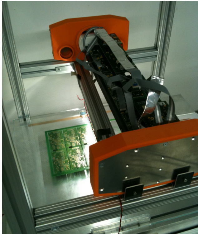
Figure 2.4: Scanner produced by Opdi-Tex GmbH for capturing image data of moving items
